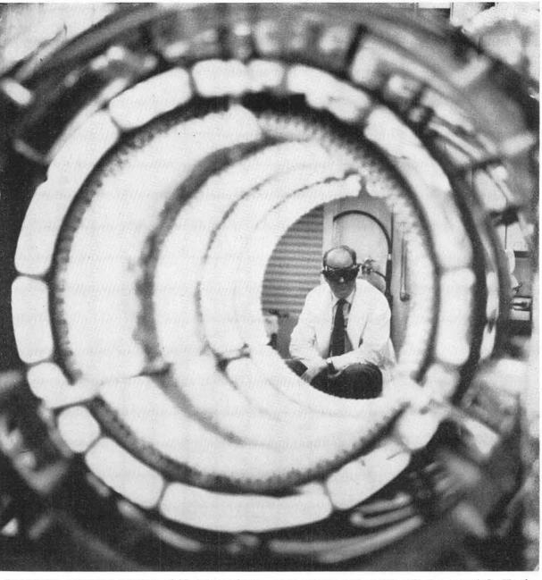
GLOWING QUARTZ LAMPS yield temperatures area where test units will be mounted. He is up to 5000° F. J. A. Barber is seen through the shown checking heater for burned out lamps.
